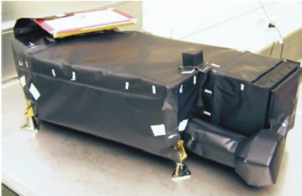
Figure 3 OSIRIS WAC flight unit (left) and optical path (right)
