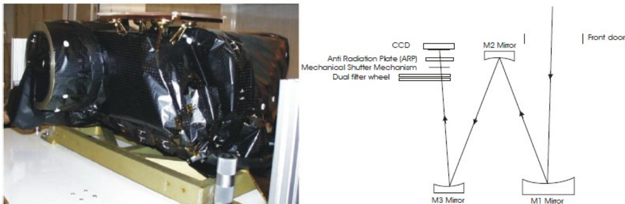
Figure 2 OSIRIS NAC flight unit (left) and optical path (right)
